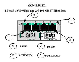
port supports fiber optic cable distances up the IEEE-standard 100Mbps distance limits, i.e., typically 2km at full-duplex and 412m at half-duplex.
